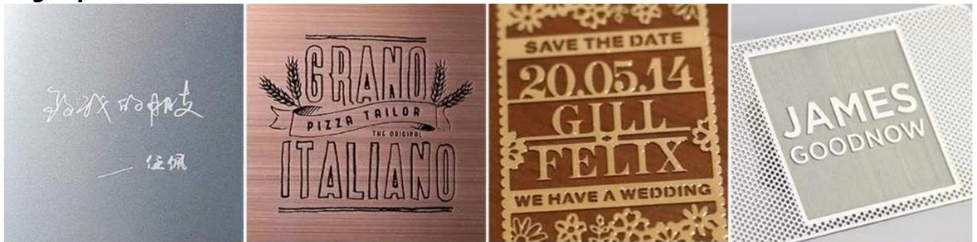
**Etch only      Etch with color infilling      Cut through      Etch reverse**
