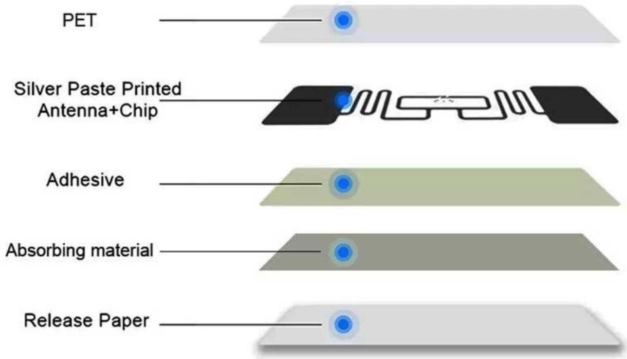
**Soft/Flexible Printable UHF Anti-Metal RFID □□ □□□□□□:**
