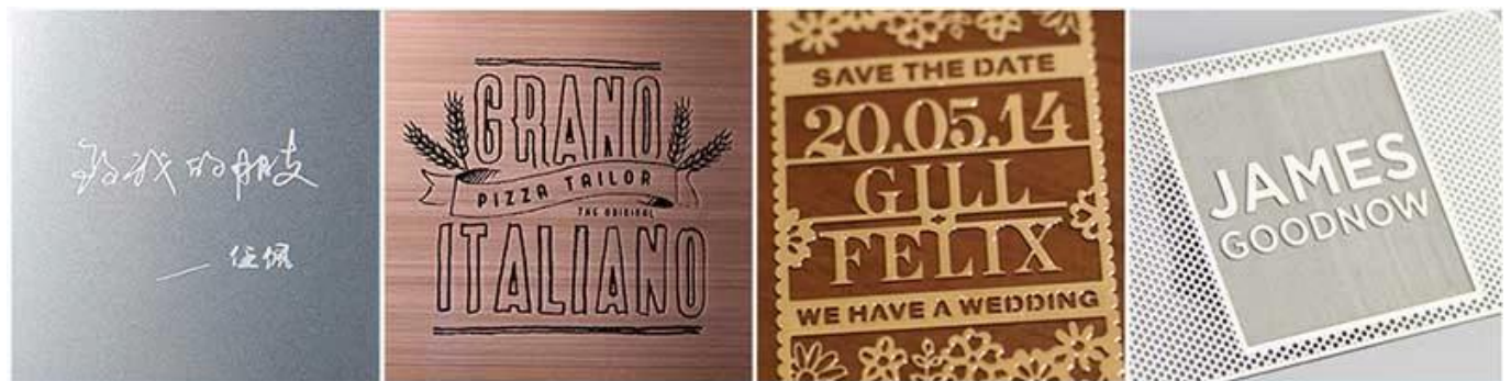
Etch only Etch with color infilling Cut through Embossed
