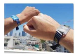
Fabric RFID bracelets are made of a fabric wristband with an RFID tag encapsulated in a housing that slides on the tape. Plastic buckle is used to secure the belt locks and can not be removed unless the wristband is cut from the cloth to remove it from the wrist. RFID tag remains readable after the fabric wristband has been cut. Optional reusable buckle the belt can easily be put on and take off.
